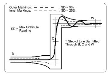
Percentage Sync - The ratio, expressed as a percentage, of the amplitude of the synchronizing signal to the peak-to-peak amplitude of the picture signal between blanking and reference white level.
